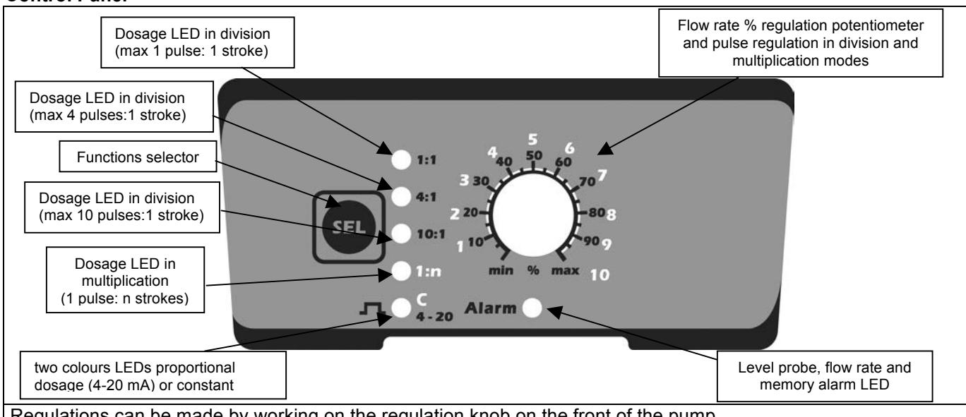
Regulations can be made by working on the regulation knob on the front of the pump
